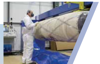
330 Gallon filament winding process
